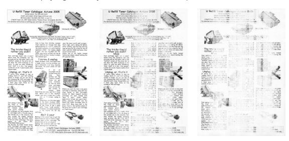
As you can see, the faded area gets wider and more pronounced with each print, but even on the last very faded page, the print at the edges is still the same blackness as on the first print. If you take out the cartridge and give it a shake at this point, perfect print will return for a few more prints – but then the fade out will return again. This pattern of progressively widening fade out bands which can be temporarily cured by shaking is the hallmark of toner exhaustion.
